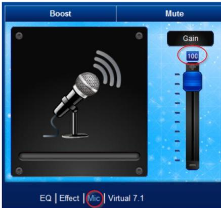
This screen allows you to set the microphone gain using the slider on the right side. You can also activate the **Boost** feature for even more recording volume.
